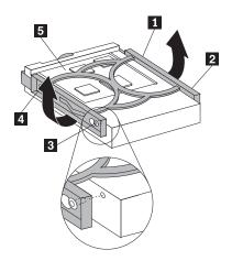
Figure 19. Installing the primary hard disk drive into the bracket
